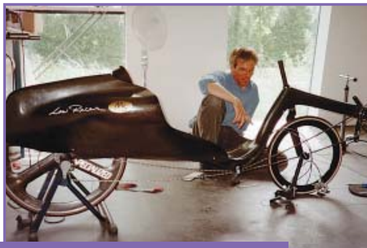
Bram Moens contemplates the carbon fibre Low Racer (the low chainline on this model precludes sharp cornering!
