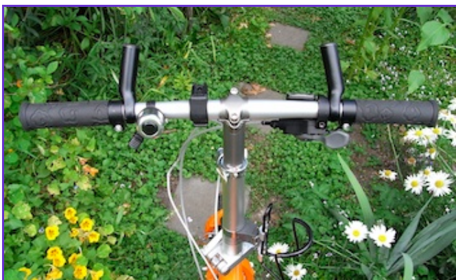
'Bar-Ins' fitted to Orange Birdy (standard 520mm bars, since taped for greater comfort)
